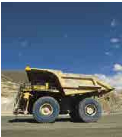
The Komatsu mining truck has a 320-tonne payload capacity.
